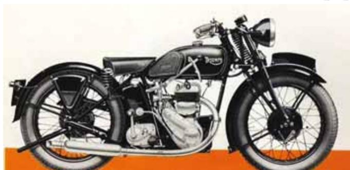
The 1935 Model 3/1 350cc (8.70 x 5.89) Side-Valve with an aluminium head looked like this when it left the factory.
